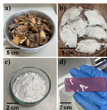
Figure 1. (a) Dried pineapple leaves, (b) extracted cellulose fiber, (c) MCC, and (d) RCS-F.
