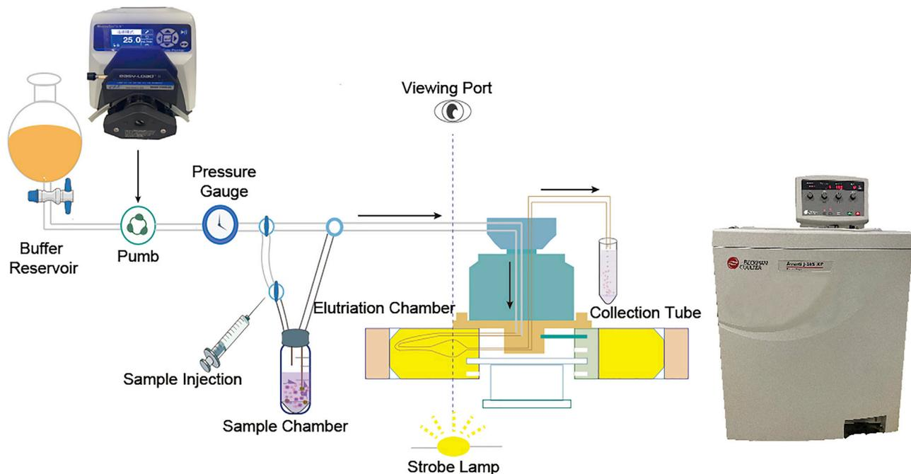
**Figure 3. Schematic diagram of the tubing pipeline connecting the buffer reservoir, sample chamber, and elutriator in the JE5.0 elutriator system (Beckman Coulter)**
