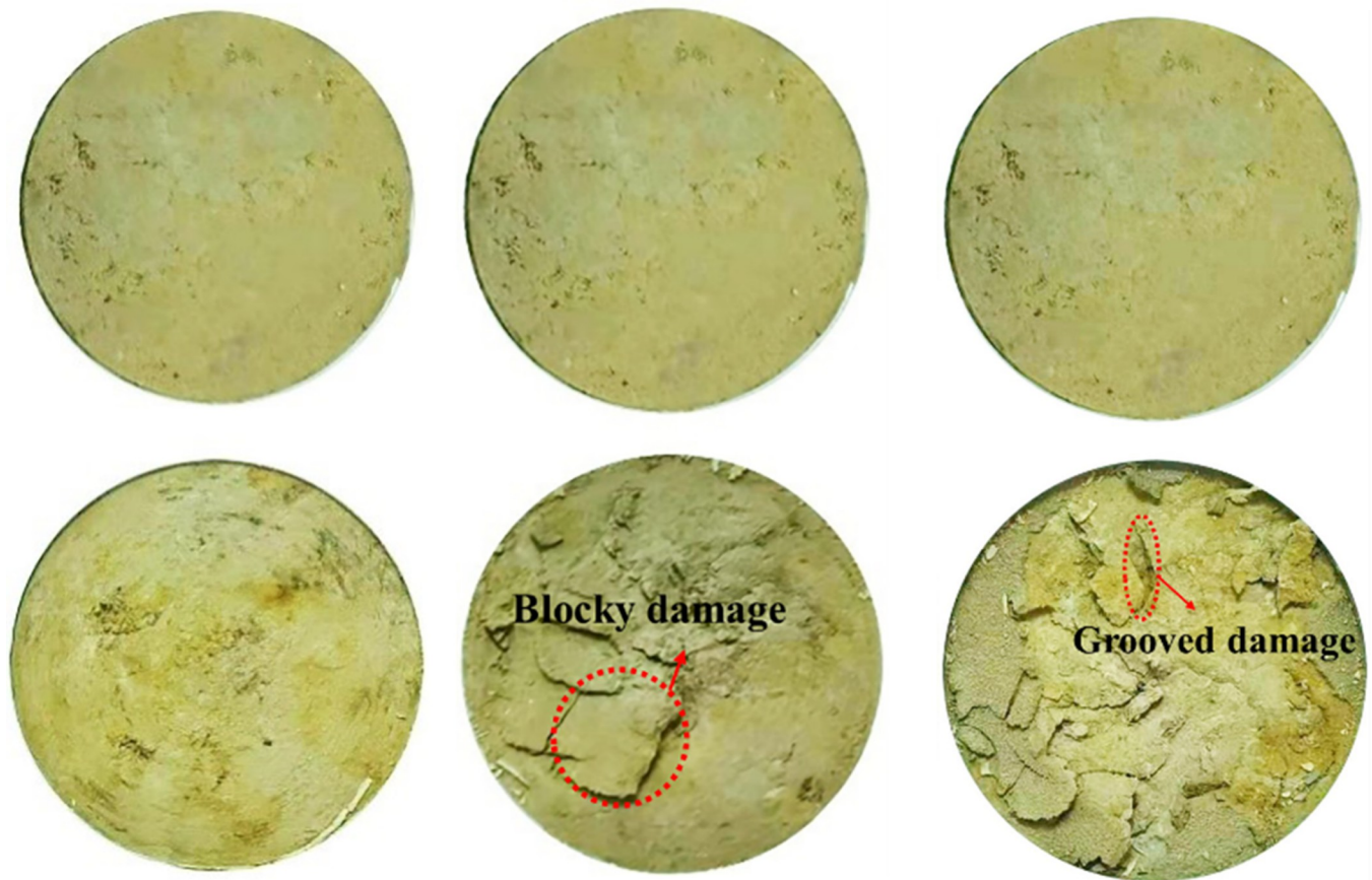
Fig 4. Comparison of the shear surface morphology of 1 # - 3 # undisturbed loess specimen before and after the test. (A) 1 # v = 0.1 mm / min. (B) 2 # v = 1.0 mm / min. (C) 3 # v = 5.0 mm / min.
