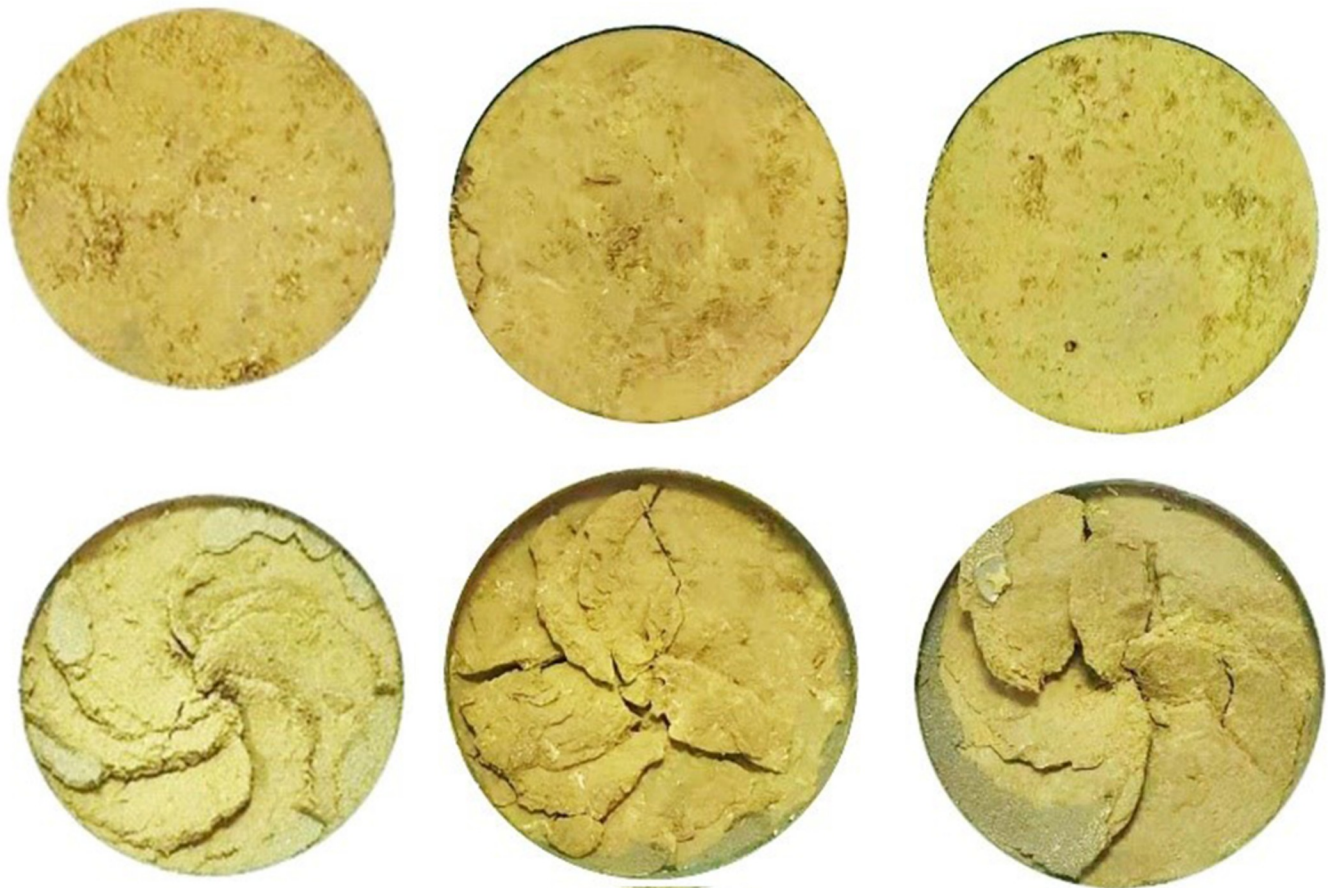
Fig 9. Comparison of the shear surface morphology of 4 # - 6 # undisturbed loess specimen before and after the test. (A) 4 # w = 16\% . (B) 5 # w = 19\% . (C) 6 # w = 22\% .
