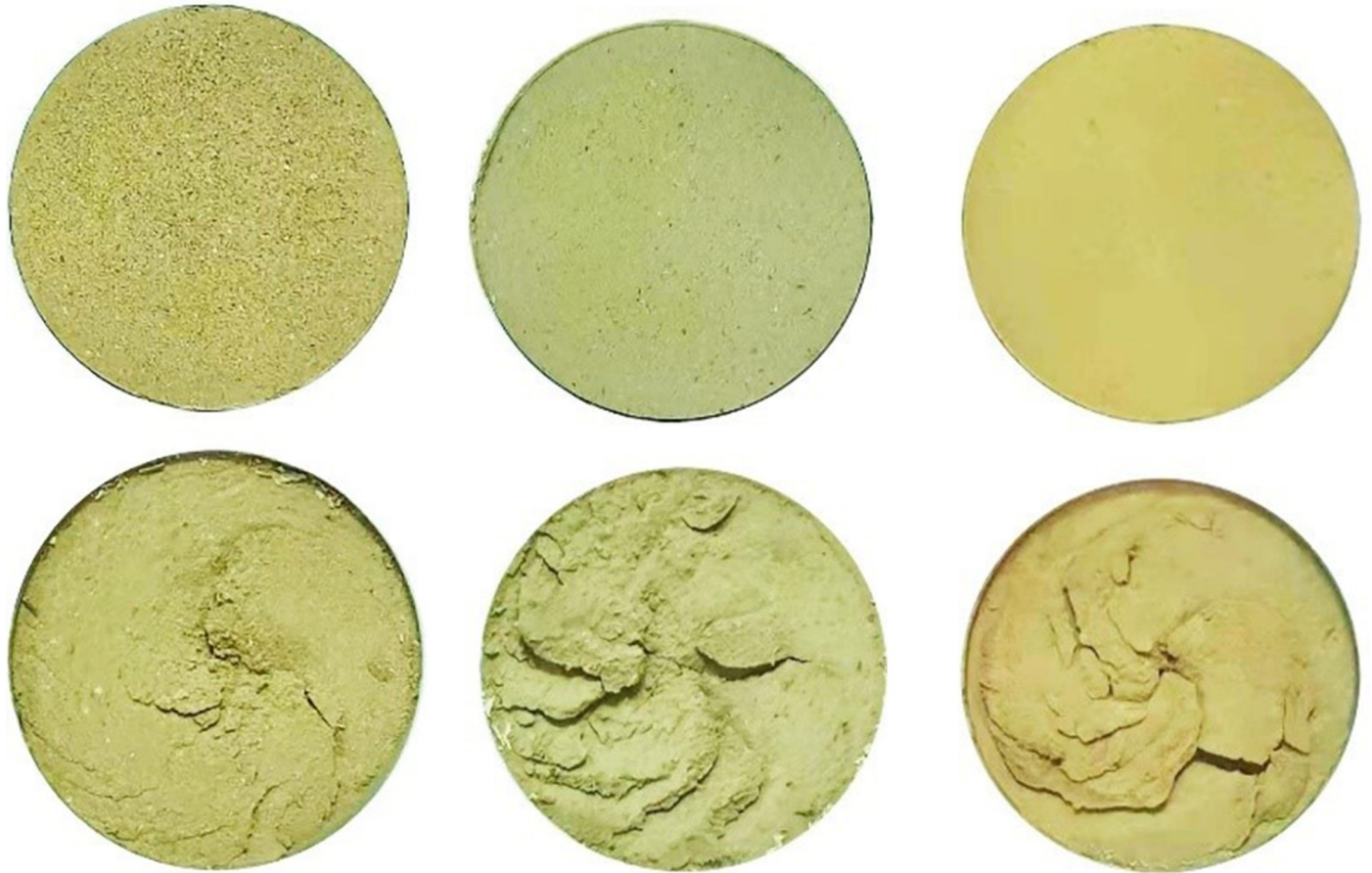
Fig 5. Comparison of the shear surface morphology of 19 # - 21 # remolded loess specimen before and after the test. (A) 19 # v = 0.1 mm / min. (B) 20 # v = 1.0 mm / min. (C) 21 # v = 5.0 mm / min.
