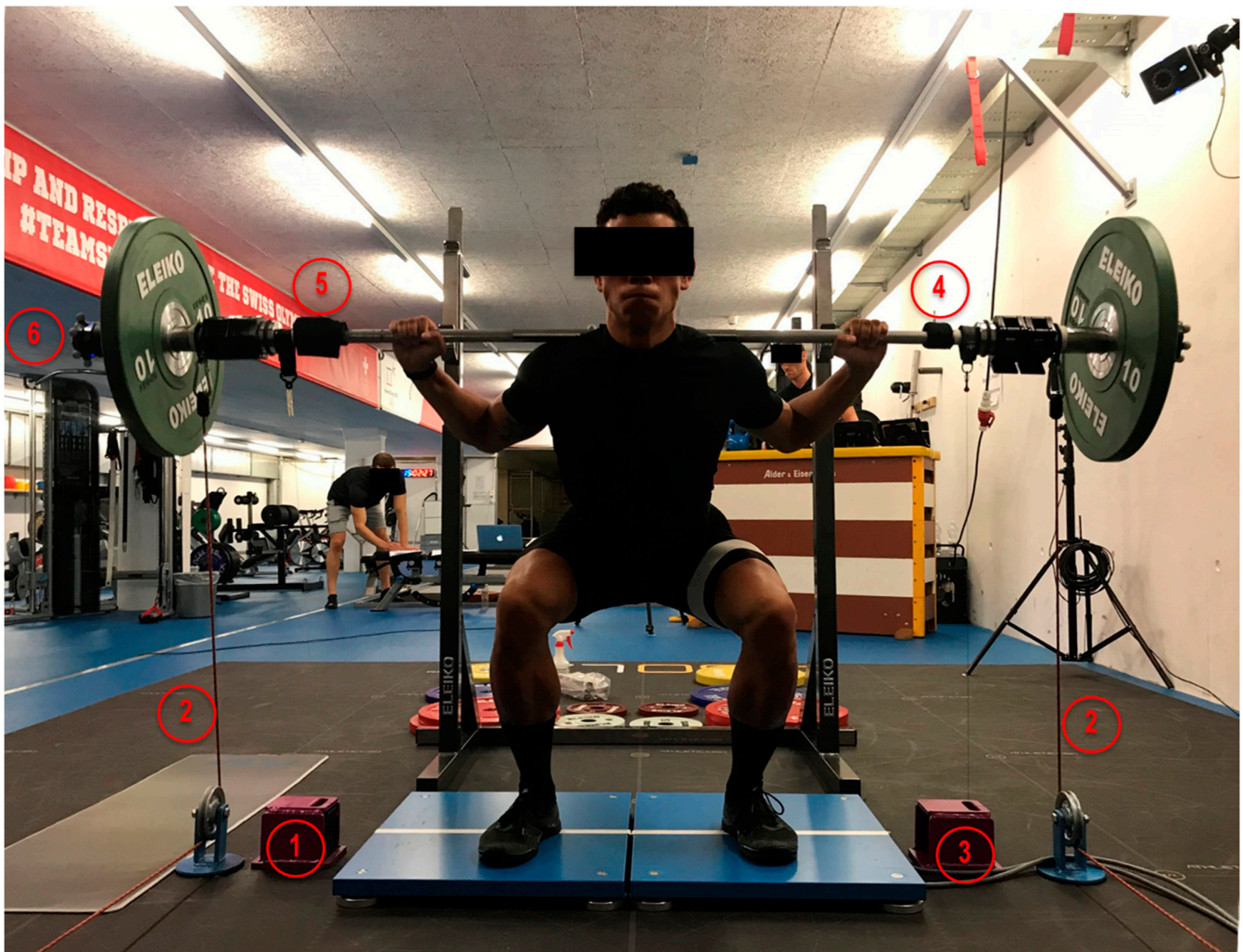
Figure 1. Study setup and locations of the tested devices on the barbell. (1) GymAware, (2) 1080 Quantum, (3) outdated linear position transducer not included in this study, (4) Vmaxpro, (5) Push, (6) Flex. A dual force plate was also in place for collecting data not addressed in the current study.
