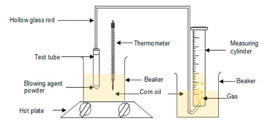
Scheme 2. Setup of apparatus.
