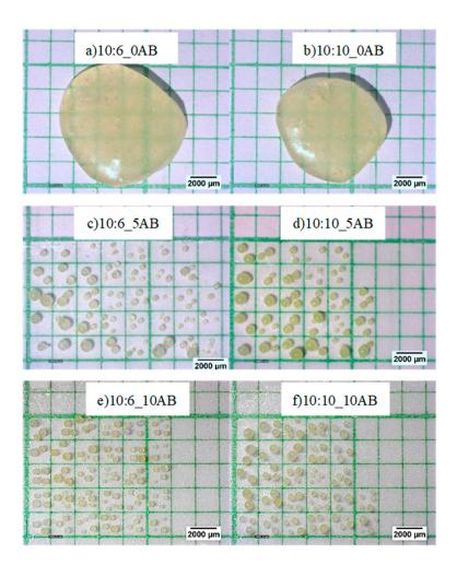
**Figure 2.** Morphology of PEMBs from a single droplet at different epoxy polyamide ratio and ammonium bicarbonate content (magnification of 20X): (a) 10:6\_0AB, (b) 10:10\_AB, (c)10:6\_5AB, (d) 10:10\_5AB, (e) 10:6\_10AB, and (f) 10:10\_10AB.
