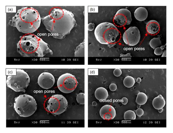
**Figure 3.** SEM images of PEMBs at different ammonium bicarbonate content and epoxy polyamide ratios at magnification of 30X: (**a**) 10:6\_5AB, (**b**) 10:6\_10AB, (**c**) 10:10\_5AB, and (**d**) 10:10\_10AB.
