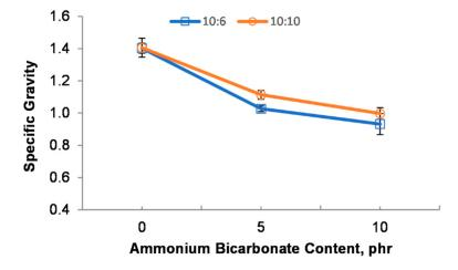
**Figure 5.** Specific gravity of PEMBs at different ammonium bicarbonate contents and epoxy polyamide ratios.
