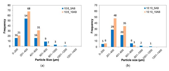
**Figure 4.** Histograms of particle size distributions of PEMBs at different ammonium bicarbonate contents and epoxy to polyamide ratios: (**a**) epoxy polyamide ratio of 10:6 and (**b**) epoxy polyamide ratio of 10:10.
