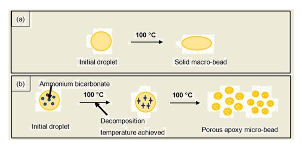
Scheme 3. Schematic illustration of the formation of PEMBs from (a) epoxy-polyamide mixture, and (b) epoxy-polyamideammonium bicarbonate mixture.
