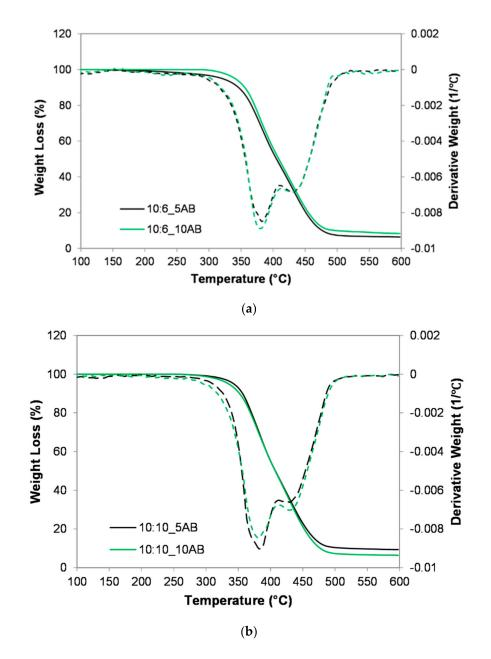
**Figure 6.** TGA thermograph of PEMBs at different ammonium bicarbonate content and epoxy polyamide ratios: (**a**) epoxy polyamide ratio of 10:6 and (**b**) epoxy polyamide ratio of 10:10.
