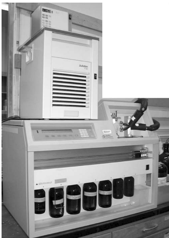
Fig. 3 Modified peptide synthesizer
