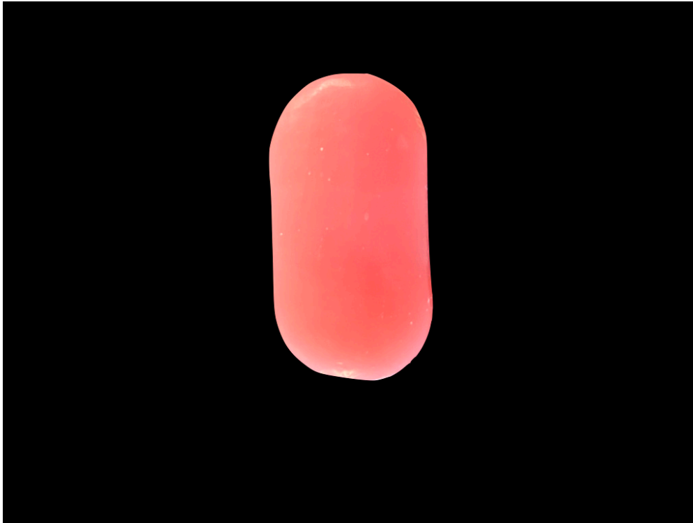
Figure 3. Polished resin sample. It shows a uniform surface with no fibers, cross linking or surface defects.
