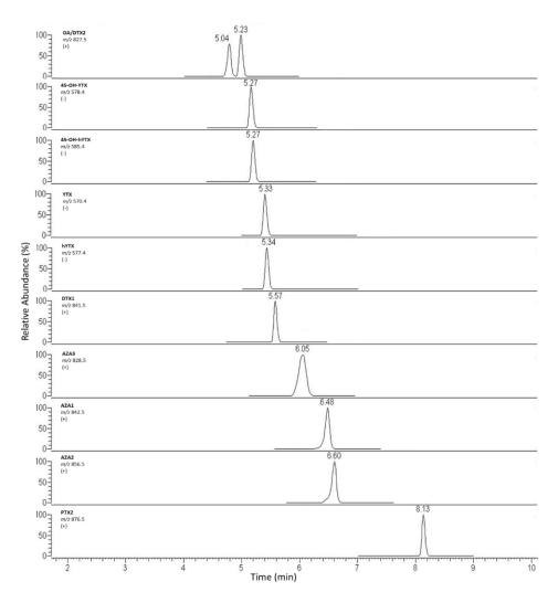
**Figure 2.** Chromatogram of mussel sample naturally contaminated with YTX toxins group, spiked with other toxins at a concentration of 160  $\mu$ g kg<sup>-1</sup>.
