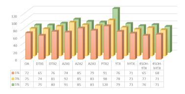
**Figure 1.** SPE clean-up optimization: comparison of three different methanolic ammonia elution solution (1%, 3%, 5% v/v).
