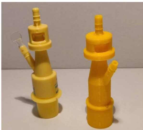
Fig. 2. Original (left) and 3D printed Venturi valves. Source: Italian hospital saves COVID-19 patients' lives by 3D printing valves for reanimation devices [61].
