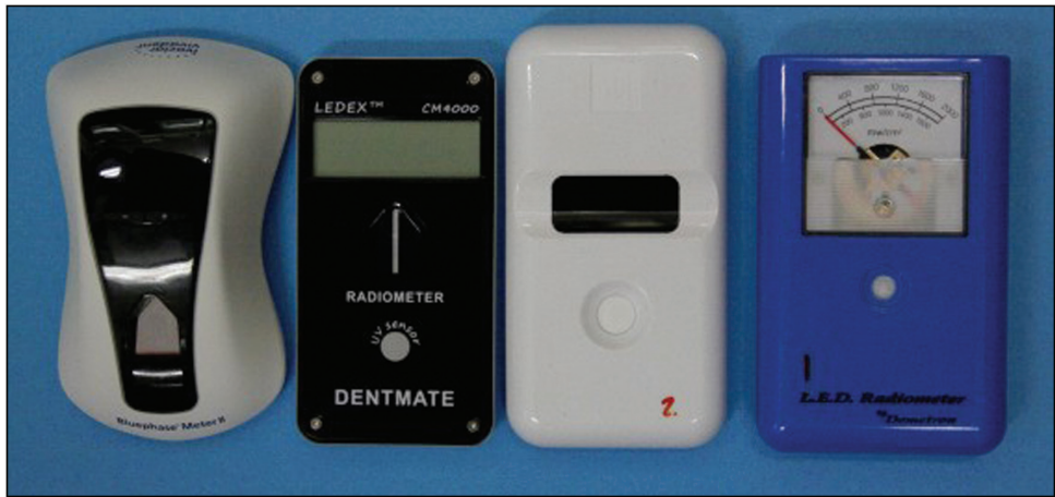
Figure 2: Two types of dental radiometers, three brands on the left are digital and one on the right is analog
