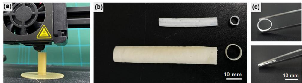
**Figure 2.** (a) 3D printing of sacrificial polyvinyl alcohol (PVA) template. (b) Cylindrical artificial vascular grafts. (c) Flexibility of the as-fabricated graft.
