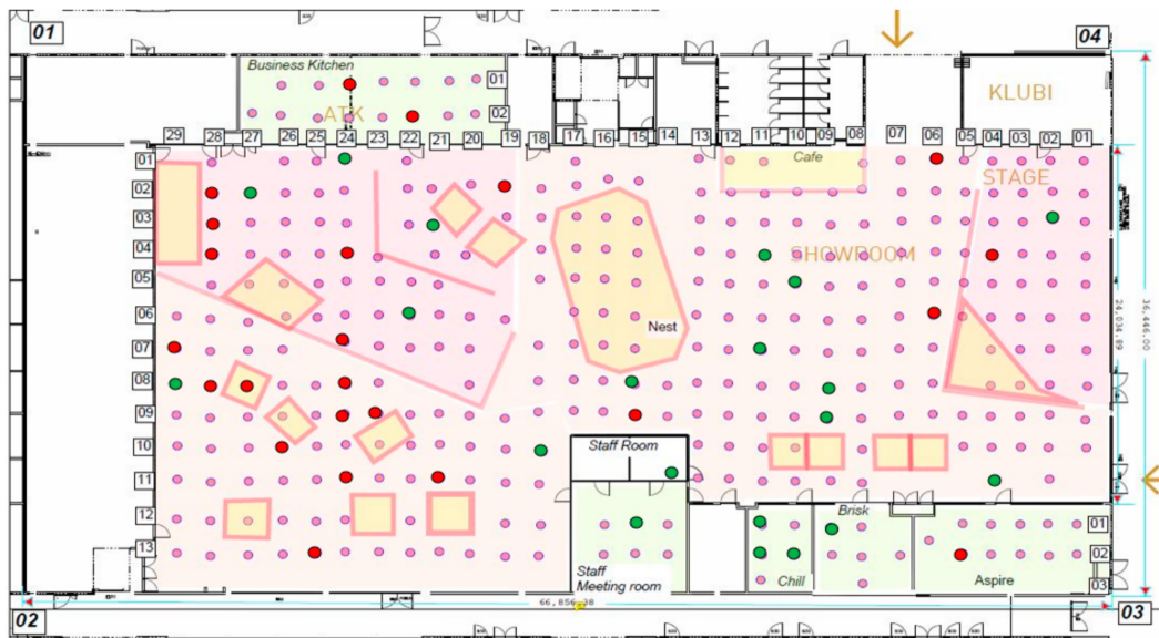
Figure 3. The floor plan showing the sensor node deployment in Tellus area inside the University of Oulu. The deployed sensors are shown as dots, distances are shown in meters, green dots indicate the sensors with the lowest packet error rate (PER) and the red dots are the ones with highest PER. Further details are provided in Section 4.
