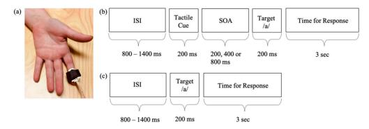
**Figure 1.** (**a**) Mechanical tactor used to deliver the tactile cues. Illustration of trials with (**b**) and without (**c**) tactile cues. ISI, Interstimulus Interval; SOA, Stimulus Onset Asynchrony.
