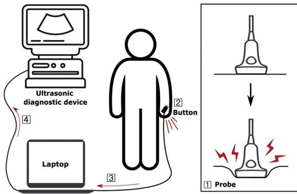
**Fig. 1.** Ultrasound imaging unit. The ultrasound imaging unit consisted of an ultrasonic diagnostic device, laptop and stop measuring button. The researcher pressed CV12 of the subject, and pressure pain occurred (1). If the button is pressed due to pressure pain (2), the button sends a stop signal to the laptop (3), the laptop sends the signal to the ultrasonic diagnostic device, and the ultrasonic diagnostic device stores the images taken so far (4).
