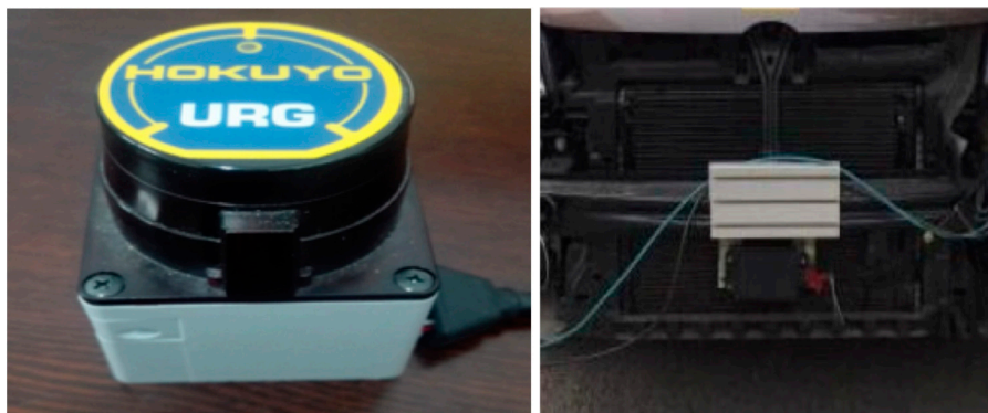
Figure 5. The URG-04LX Lidar (Left) and the ESR Radar (Right).
