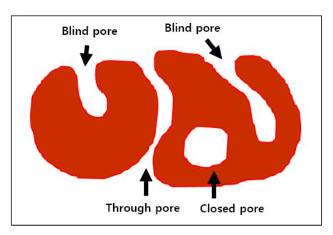
**Figure 2.** Pore classification by physical shape (Total porosity = Open-pore porosity + Closed-pore porosity; Open-pore porosity = Through-pore porosity + Blind-pore-porosity).
