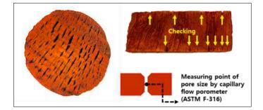
**Figure 5.** Checking of delignification-treated red toon and measuring point of pore size by capillary flow porometer.
