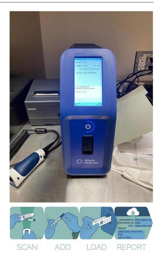
**Fig 1. A.** Diagnostic Analyzer for Selective Hybridization (DASH) PCR machine at point-of-care in clinical space. **B.** Diagnostic Analyzer for Selective Hybridization (DASH) PCR machine workflow: barcode on cartridge scanned, nasal swab added to cartridge and snapped at break point, cartridge loaded into DASH machine, and report generated on screen/printed after approximately 15 minutes.
