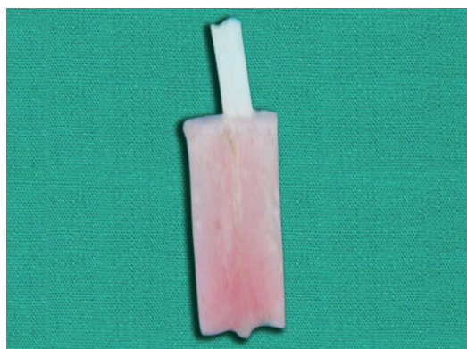
Fig. 2: Glass fiber post pieces were embedded horizontally in the center
