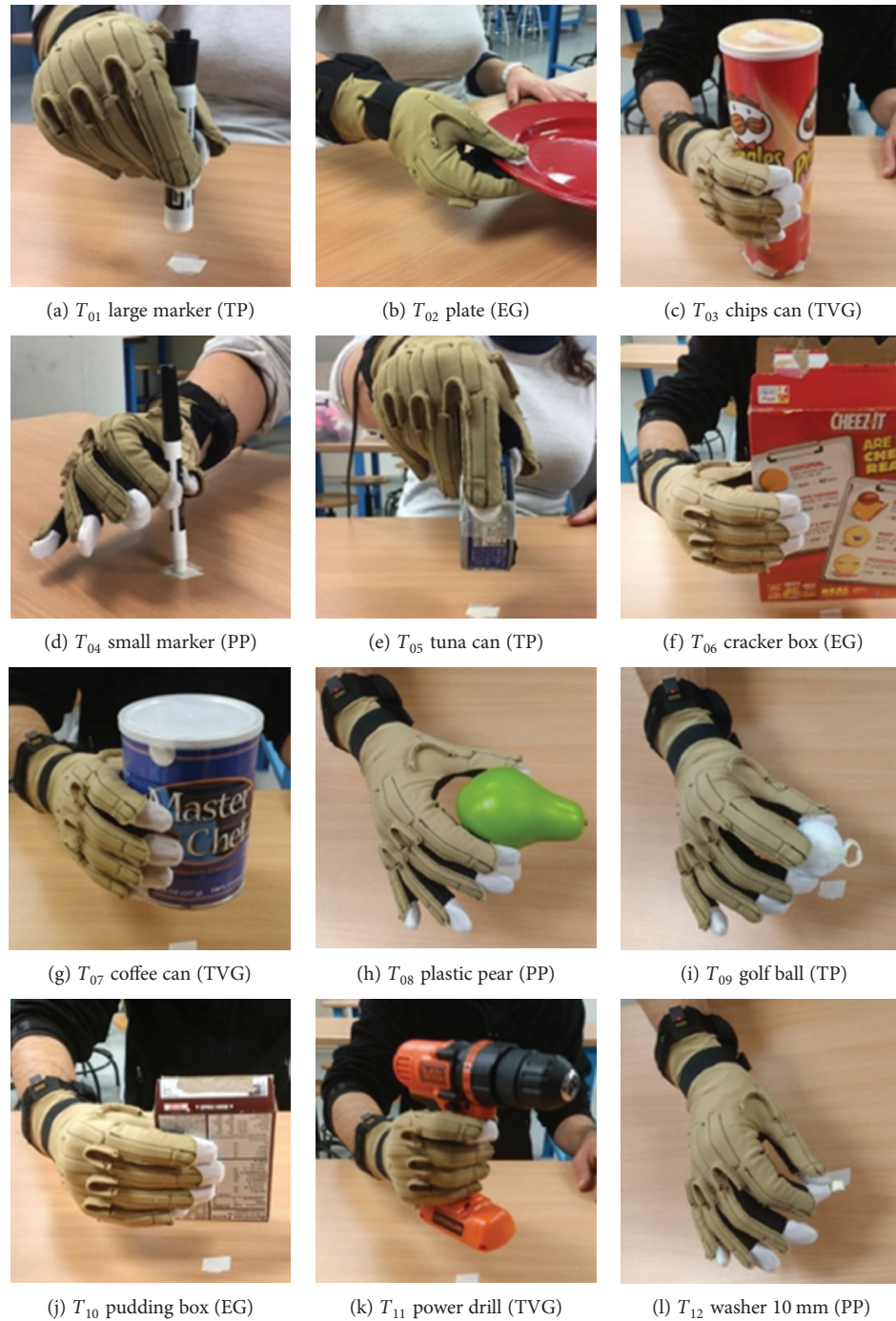
FIGURE 2: Grasping tasks of the experiment (a-l). T_g are the tasks ordered ( g : indicates the order) followed by the object of the Yale-CMU-Berkeley Object and Model Set [14] to grasp and in brackets the grasp type to be performed in each task (TP: tripod pinch, EG: extension grip, TVG: transverse volar grip, and PP: pulp pinch).
