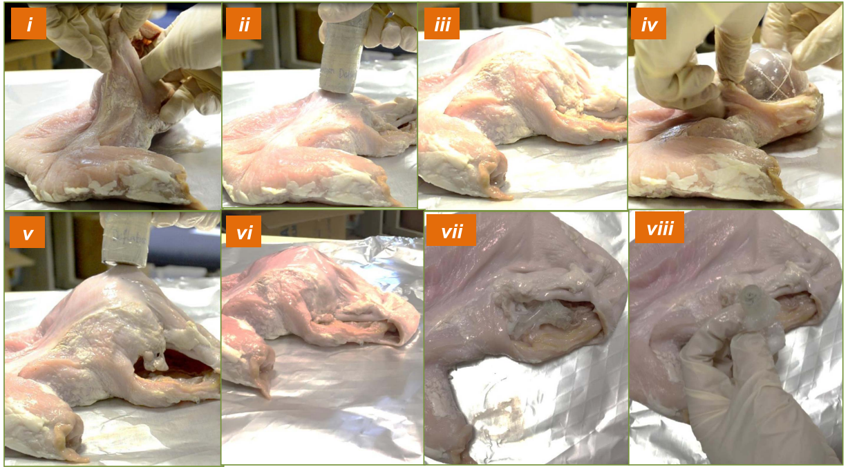
Figure 6. Validation on a fresh porcine stomach; (i) Insert the capsule-balloon into the porcine stomach; (ii) Introduce the external magnet to the porcine stomach; (iii) Chemical reaction and balloon is fully inflated; (iv) The inflated balloon is partially exposed from the porcine stomach for observation; (v) External magnet is introduced again for the balloon deflation; (vi) Deflation valve is opened and balloon is deflated; (vii) Balloon is completely deflated; (viii) Deflated balloon and its inner capsule are removed from the porcine stomach.
