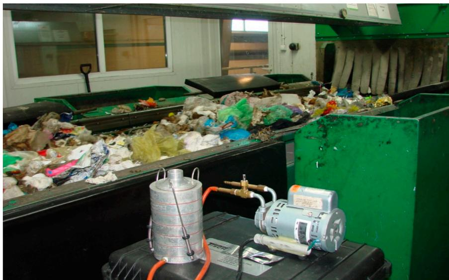
**Figure 2.** Six-stage Andersen impactor used during measurements in a waste-sorting plant located in Southern Poland.
