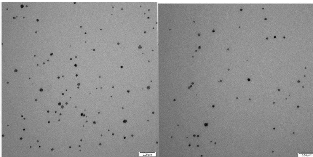
**Fig. 1.** Particle Characterization: Transmission electron micrograph (TEM) of chitosan coated 5 nm particles. One-hundred particles were measured to determine the average primary size to be  $3 \pm 1.2$  nm.
