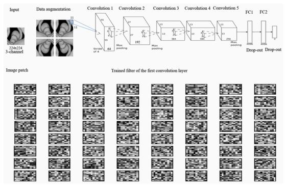
**Figure 2.** The proposed convolutional neural network consisting of convolutional layers, max-pooling layers, fully-connected layers, drop-out layers, and final layers of classification. The number of filters, the connections in each layer, and the first layer of the learned convolutional kernel are described above. FC, fully-connected.
