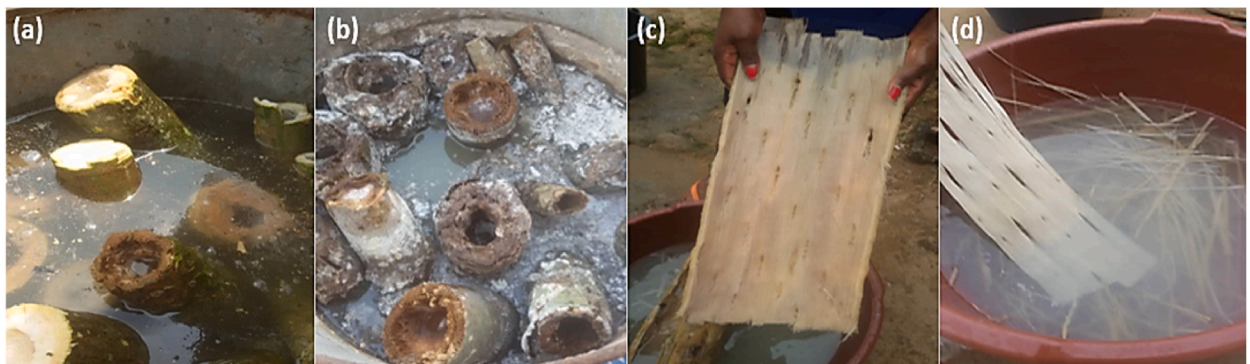
Fig. 1. Stagnant water extraction; (a): Submerged papaya trunk; (b): Decomposing trunks; (c): Fiber mat; (d): Mat submerged in water.
