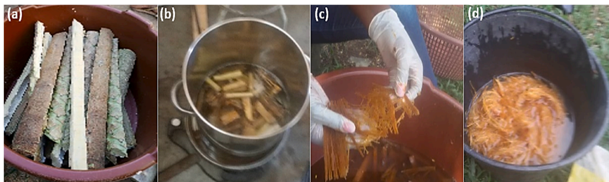
Fig. 2. Extraction with NaOH; (a): Pieces of carica papaya pseudostem; (b): Pieces of pseudostem immersed in NaOH; (c): Extraction of fibers; (d): Rinsing of extracted fibers.
