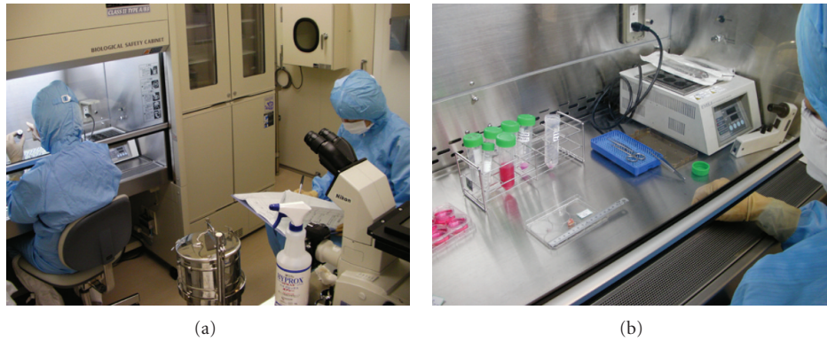
FIGURE 2: CPC of Tokyo Women’s Medical University. (a) Individuals who work in the CPC wear sterile clothing, gloves, caps, and masks to avoid releasing possible contaminants. (b) All tubes and dishes were labelled to avoid misidentification.
