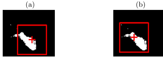
Fig. 3. ROI centroid positions: (a) Original centroid and (b) Adjusted centroid.
