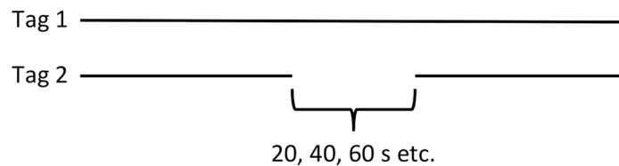
Fig 2. A. Illustration of a staggered log. One tag records for at least one additional pulse. In this study, the pulse rate was set at 20s. B. Illustration of a broken log. One tag records two separate logs while the other in the dyad records one continuous log.
