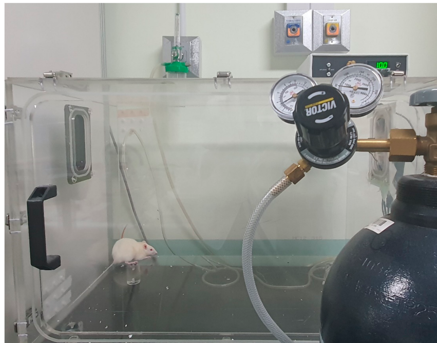
Figure 1. Hypoxic chamber with 10% oxygen. Animals sojourned for 2 ( n = 10 ), 4 ( n = 10 ), and 8 h per day ( n = 10 ) in one identical commercially designed chamber ( 30 \times 320 \times 320 inches) for five days. Deviations from the desired concentration were corrected by the addition of N_2 through solenoid valves.
