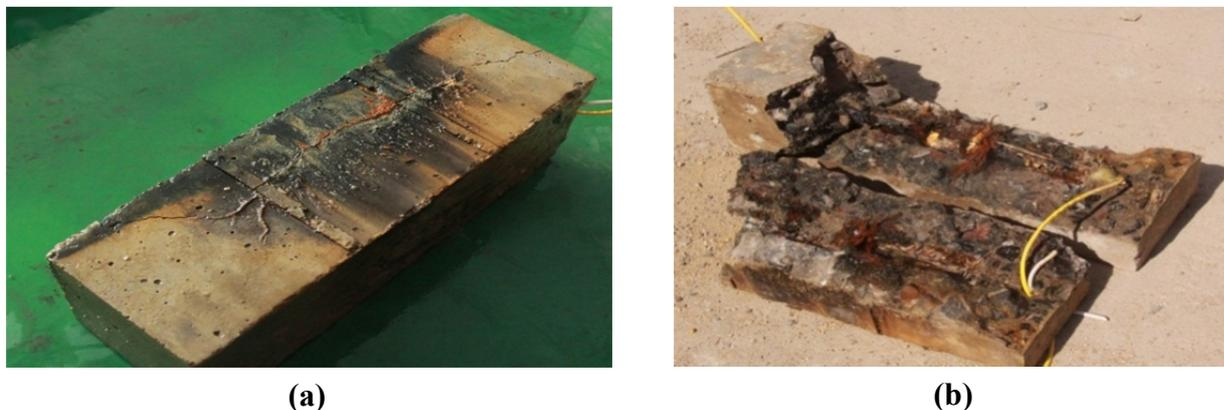
The improvement plan of BCES-III is to remove the porous material layer of the sensor or reduce its thickness so as to increase its sensitivity of the steel corrosion monitoring, or to replace the PTFE material with some other kind of material with better compatibility. Meanwhile, it is better to apply the sensor to monitor serious corrosion conditions.
