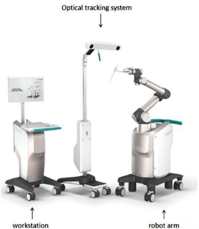
Fig. 1 TiRobot, mainly composed of a workstation, an optical tracking system, and a robot arm (Photo provided by Beijing Tianzhihang Medical Technology).
