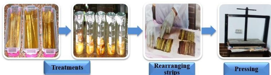
**Figure 2.** Papyrus strips treated with different treatments and sheet formation by lamination, then cold pressed.
