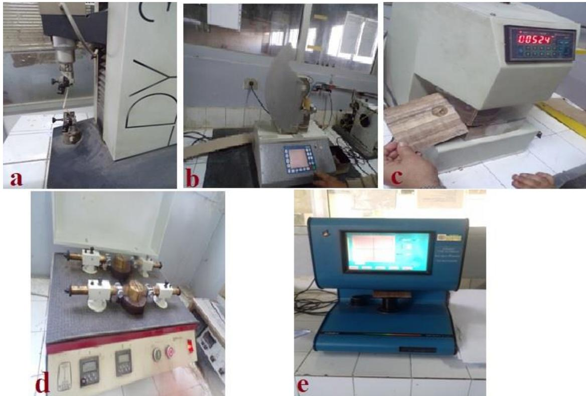
**Figure 4.** Apparatuses for measuring the mechanical and physical properties of the manufactured papyrus sheets. (a) Tensile testing machine; (b) Tear testing machine; (c) Burst strength tester BS 20T; (d) Double-fold number DBF 6-60; (e) Spectrophotometer Color.
