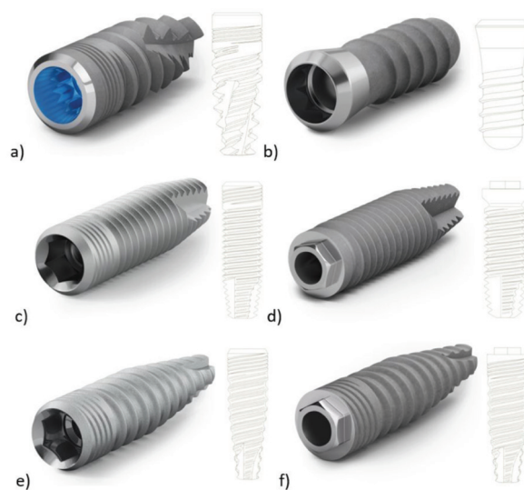
Fig. 1: Images of the implants used in the present study. a) M12: Morse taper connection, aggressive tapered profile, Grade IV titanium; b) M8: Internal octagon connection, less aggressive cylindrical profile, Grade IV titanium; c) L35: Internal hexagon connection, cylindrical profile, Grade V titanium; d) L6: External hexagon connection, cylindrical profile, Grade V titanium; e) N35: Internal hexagon connection, tapered profile, Grade V titanium; f) N6: External hexagon connection, tapered profile, Grade V titanium.
