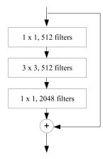
Fig. 2 A building block in conv5 of ResNet-101.
