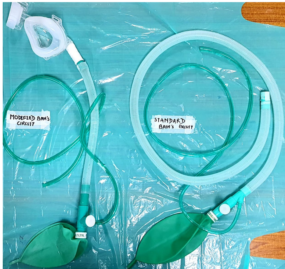
FIGURE 1: On the left is a modified Bain's circuit with reduced length and attached NIV mask, on the right is a standard Bain's circuit
