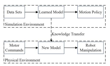
Figure 4. Principle of transfer learning for robot manipulation.
