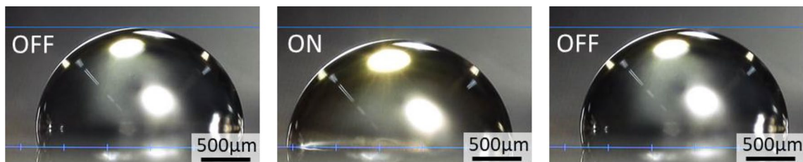
Figure 5. Experimental results of height control of a droplet by electric field for EWOD. A 4 \mu\text{l} DI water droplet is prepared on a circular pattern for a droplet. Side views of the droplet are observed as the applied voltage is turned off and on. The height of the DI water droplet is successfully decreased through the application of an electric field. The height of the droplet, which is 1290 \mu\text{m} in the initial state, decreases to 1101 \mu\text{m} when a voltage of 160 V is applied, as shown in this figure. The height of the droplet increases when the applied voltage is turned off.
