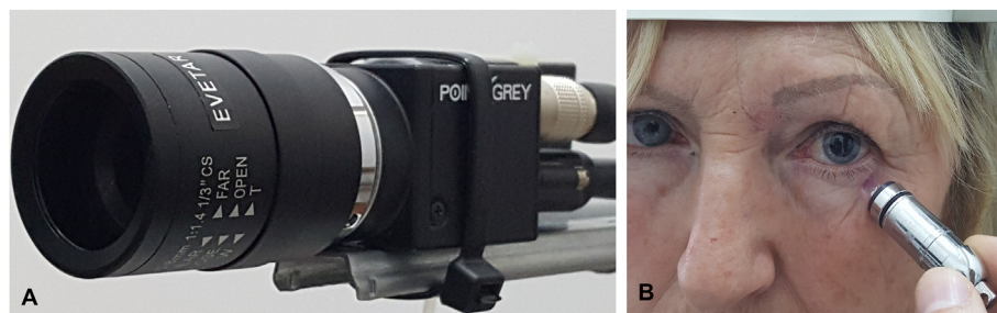
Fig. 2. A. The device for transpalpebral NIR transillumination. B. The wireless near-infrared (940 nm) LED probe position during examination with the transpalpebral approach.
