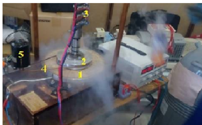
Figure 21. Prototype under tests: (1) inductor, (2) stator, (3) brushes and rings, (4) transmission belt, (5) synchronous motor.
