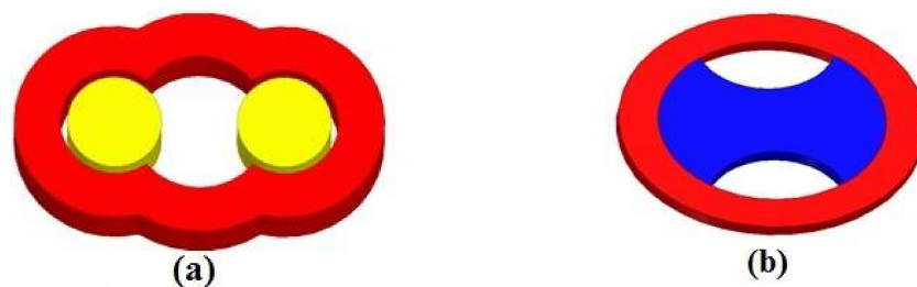
Figure 8. New kind of superconducting inductors: (a) inductor with optimized coil, (b) inductor with optimized YBCO plat.
