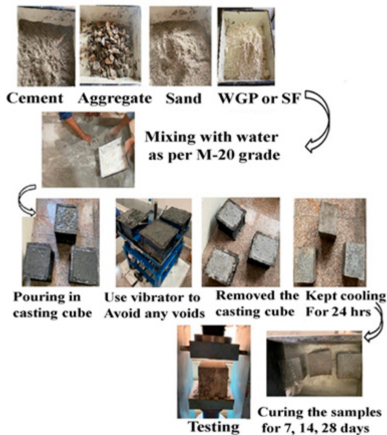
Figure 3. Process of formation of green concrete through the waste.
