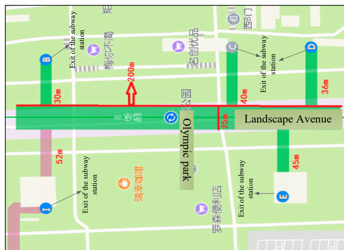
(b) Two-dimensional planar structure of subway station.
