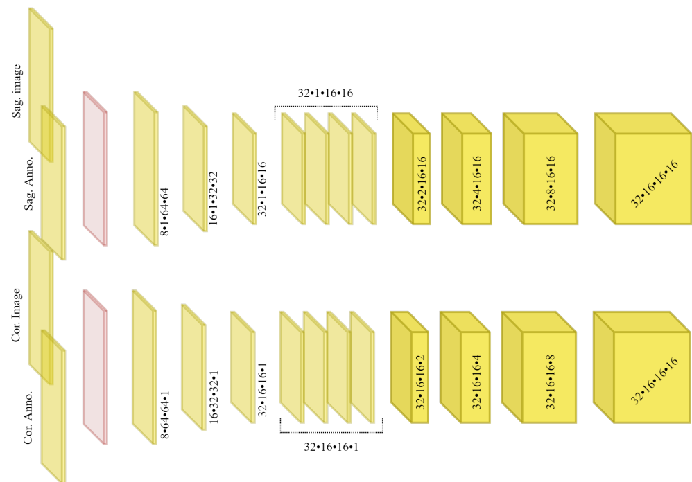
Figure 5. Architecture of the orthogonal encoders, which employ anisotropic convolutions, with an anisotropy along the dimensions that need to be expanded. We use ‘squeeze and excitation’ blocks (depicted in red) to fuse the image features and annotation features.
