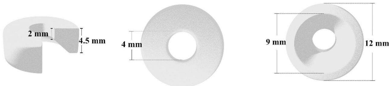
Fig. 1 The three-dimensional structure of ring magnet for magnet-assisted diverticuloplasty
