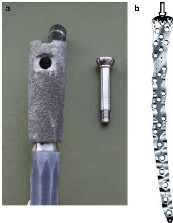
Figure 4. (a) Photograph of lateral view of a proximal Arcos hip prosthesis with reattachment bolt and (b) Zimmer noncontact bridging plate with arrow indicating the hole that was enlarged in the plate.
