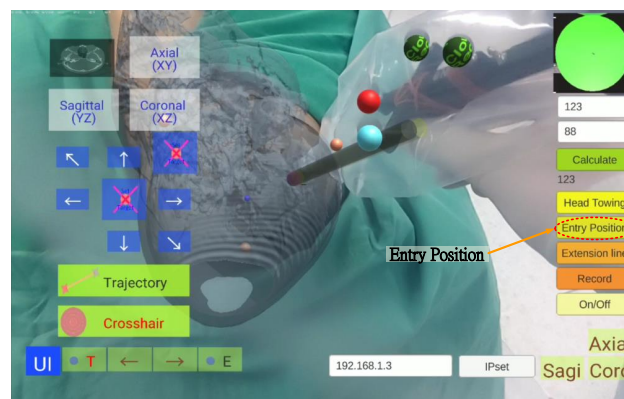
Figure 12. Entry point position setting.
