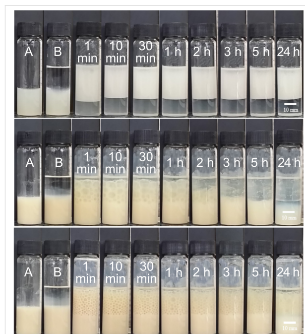
Figure 4: Photos of vessels containing cyclohexane-in-water emulsions stabilised by particles of \text{Ce}_{0.495}\text{Sn}_{0.495}\text{Pd}_{0.01}\text{O}_{2-\delta} at concentrations in water of 0.03 wt % (upper), 0.30 wt % (middle) and 1.0 wt % (lower) at different times since preparation. A is the aqueous dispersion of particles, B is after addition of oil but before emulsification.
