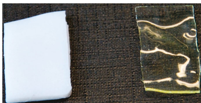
Figure 11. Poly(GL-co-4MeCL) (75:25) before (left) and after (right) thermal cross-linking with dicumyl peroxide. Reprinted with permission from [131]. Copyright (2011) American Chemical Society.
