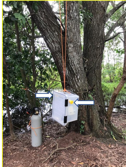
Figure 2. CO 2 -baited SMACK trap housing two honey-baited FTA™ cards (arrows).
