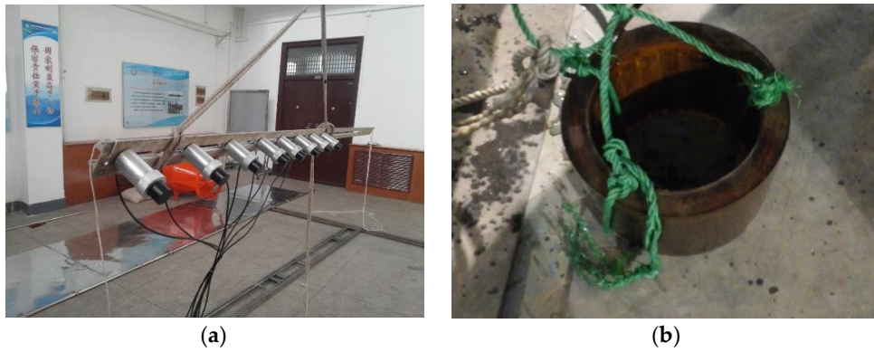
Figure 8. (a) The hydrophone array (b) The underwater acoustic transducer.
