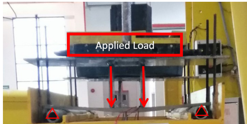
Figure 4. A coupon sample under four-point bending creep.
