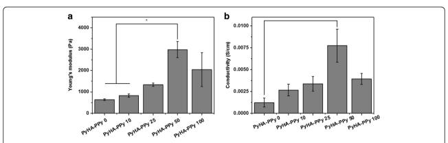
**Fig. 2** Mechanical and electrical properties of the PyHA-PPy hydrogels. **a** Young's modulus of the fabricated hydrogels. **b** Conductivity of the fabricated hydrogels. Averages and standard deviations were plotted (n=3). Statistical difference was assessed using the student t-test and statistical significance was denoted with an asterisk (p < 0.05)
